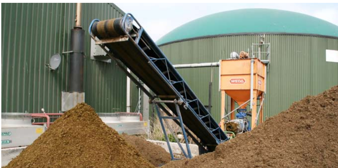
Fibres of digestate used for animal bedding after drying
